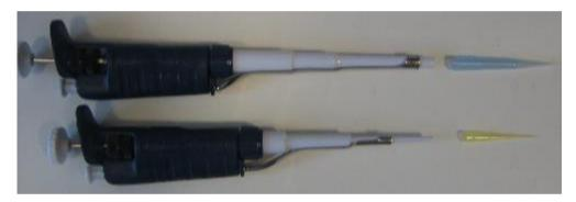
Before fitting the tip adjust the reading on the side to reflect the amount you want to pipette by twisting the black nut or white head in the appropriate direction. The numbers are read from the top towards the tip and reflect different values depending on the size of pipette being used.
